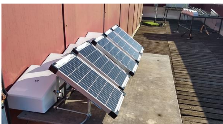
Figure 1: Endurance test of our IoT sensor box for measuring air quality
