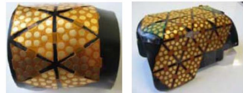
Fig. 2: An example of e-skin using flexible printed circuit boards 2 .
