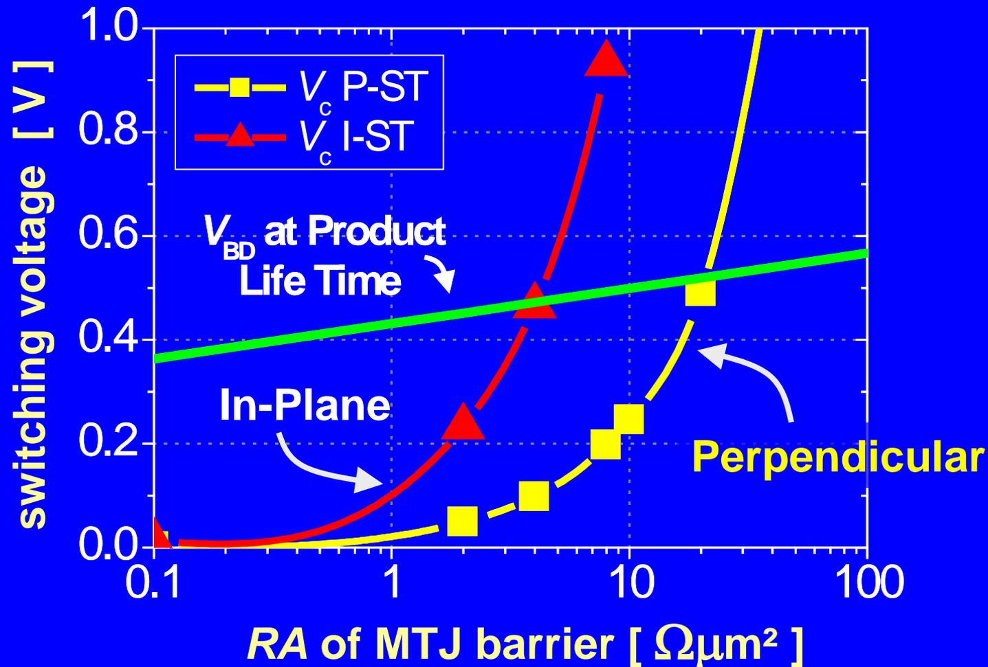
⇒ P-ST allows to use high RA for reliable operation
