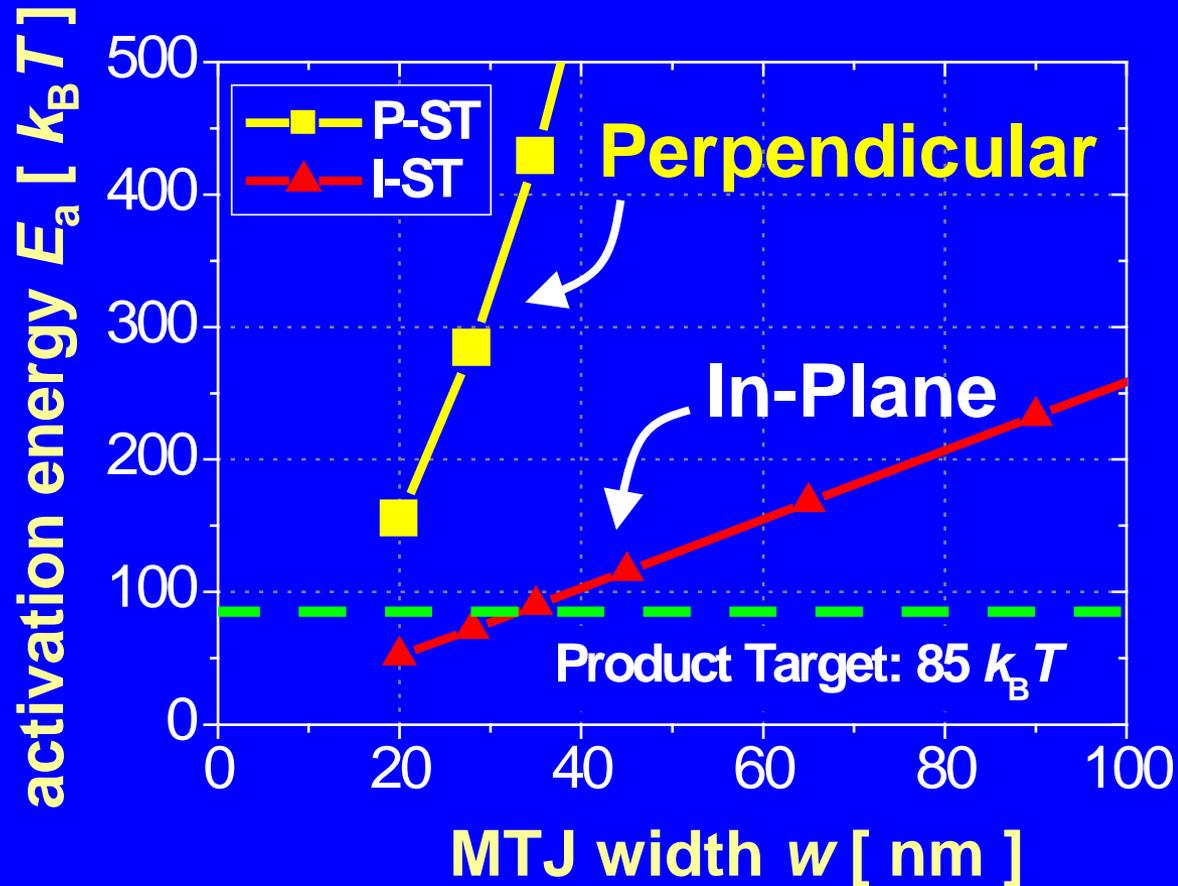
High anisotropy ensures scaling below 20 nm
