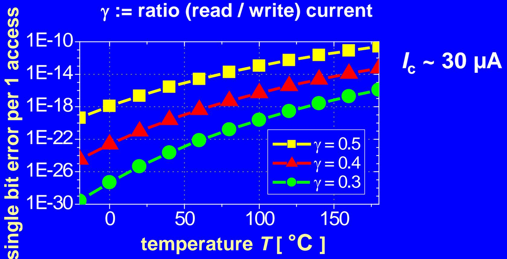
↪ At  $I_c \sim 30 \mu\text{A}$  a read current of  $I_r \sim 10 \mu\text{A}$  ( $\gamma \sim 0.3$ ) is feasible without read disturb
