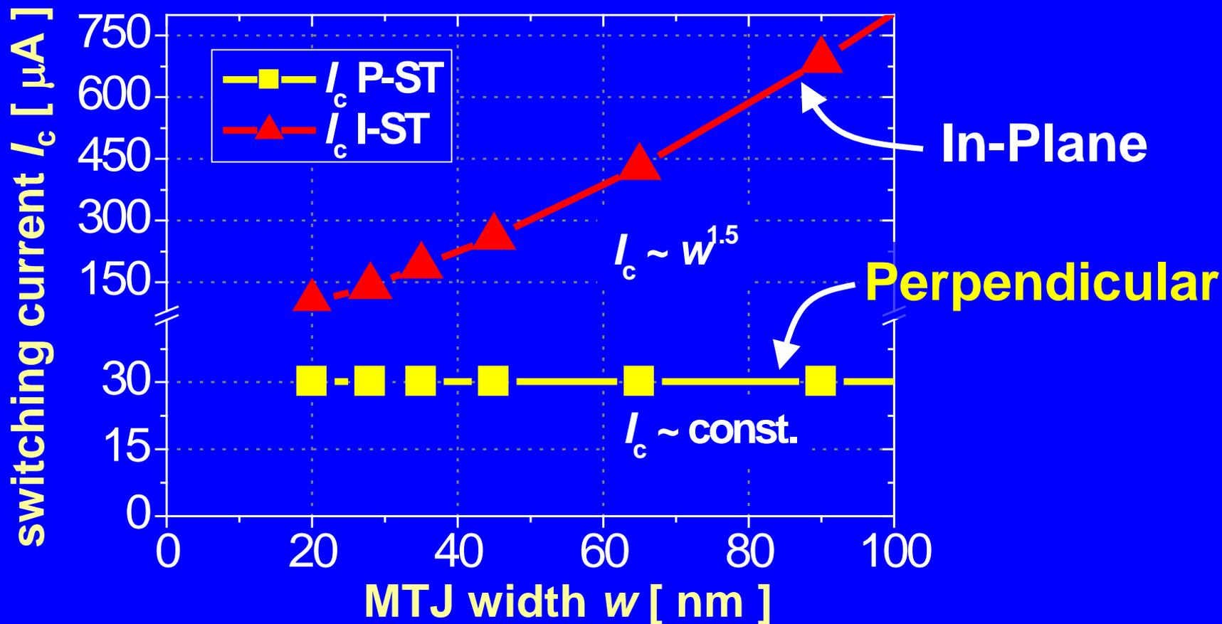
↪ Absence of demagnetization fields reduces required switching current  $I_c \sim 30 \mu\text{A}$
